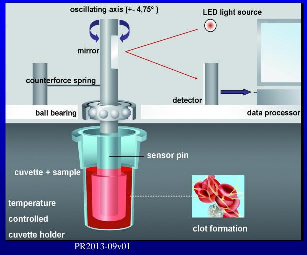
ROTEM's shaft, spring, and ball bearing technology detects clot formation and uses an inverse function to display a tracing that resembles clot formation. It is less susceptible to movement or vibrations that can affect other viscoelastic methods.
