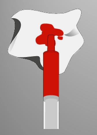
Any air bubbles in the sample must be expelled as soon as possible after the sample has been drawn
